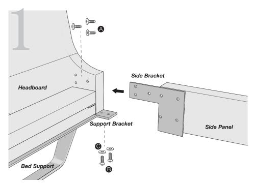
Secure Side Panel on Headboard with Flathead Allen Screws(A) and Button Head Screws(B)/Washers(C). IMPORTANT: Tighten Side Bracket to Headboard first, then tighten Support Bracket. Repeat on opposite
