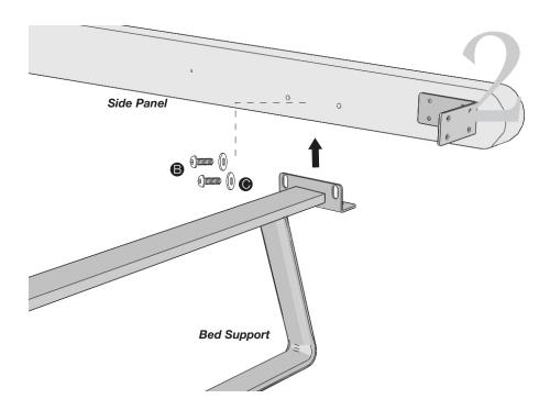
Slide Bed Support under both Side Panels and secure with Button Head Screws(B)/Washers(C). Repeat on opposite side. NOTE: Do not tighten until fully assembled.
