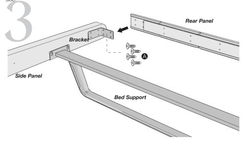
Align Rear Panel onto the Side Panel Bracket. Secure with Flathead Allen Screws(A). Repeat on opposite side. Tighten all screws to complete bed assembly.
